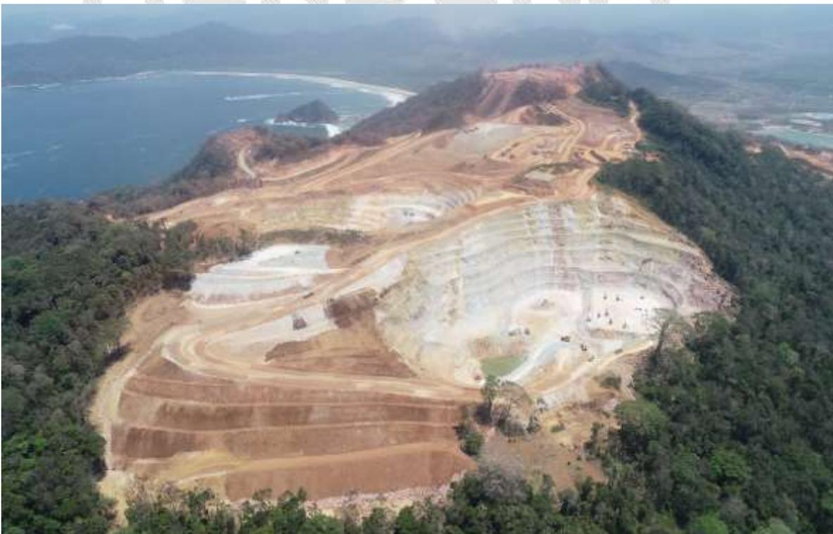
Figure 3 – Open Pit Mining - Pit A showing cutback 1 in foreground and Dam 1 in the background.
