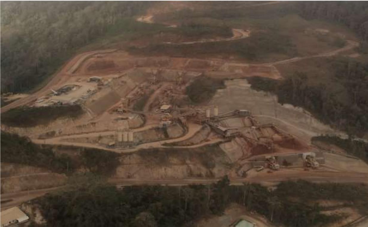
Figure 6 – Aerial view of the Heap Leach Pad showing Lift 4 Expansion
