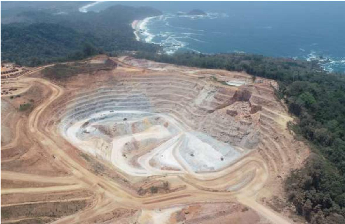
Figure 2 – Open Pit Mining - Aerial view of Pit B East cutback 2 in foreground and Pit A & Pit C In the background.
